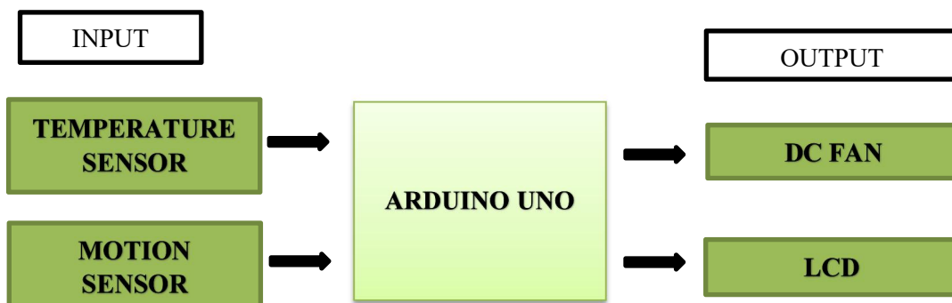
Figure 3.1: Block diagram of project operation
