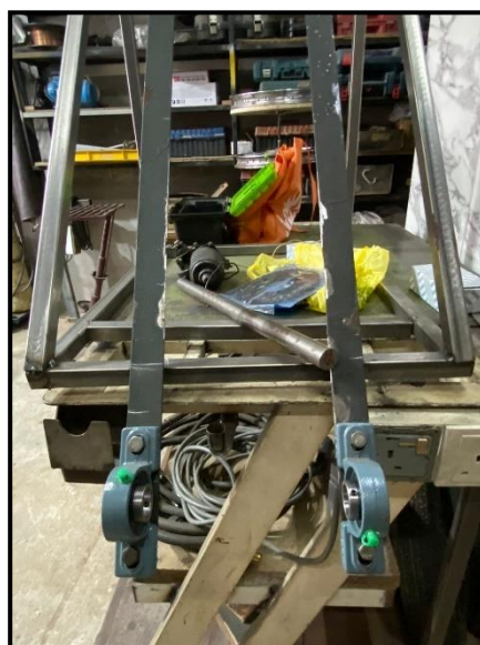
Rajah 25 Pemasangan 4 Set Bearing
