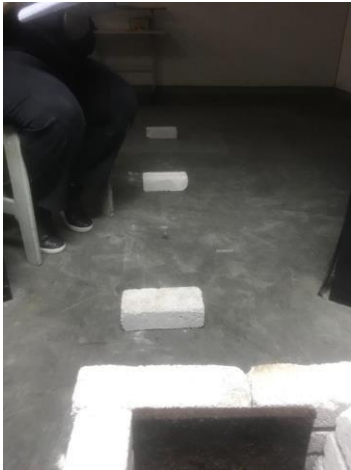
Figure 3.11 : The arrangement of brick (sound source)
