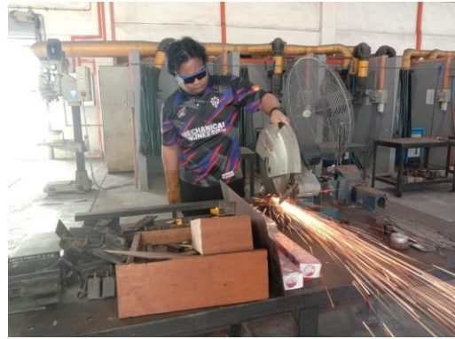
Figure 6.3 Cutting the Hollow Steel
