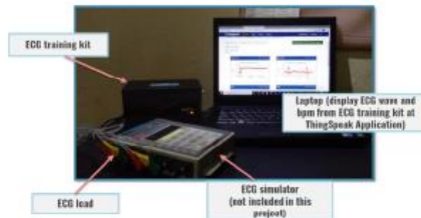
Figure 7: ECG Training Kit System with IoT via ThingSpeak Application
