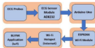
Figure 2: Flow diagram of ECG Monitoring Healthcare System
