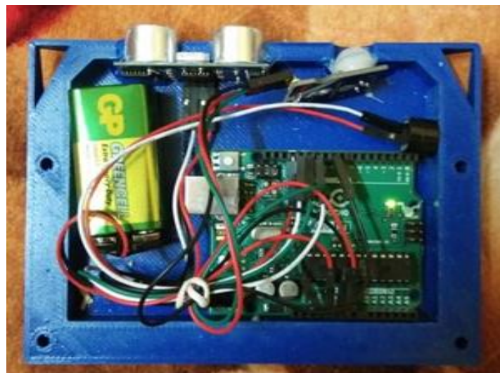
Figure 4.2.2.2 Arduino Board and Sensor in The Case.
