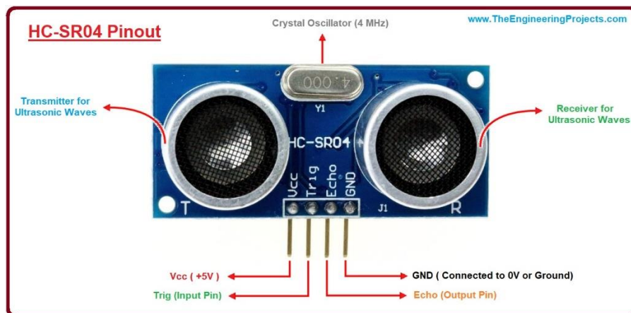
Figure 3.2.2 (k) HC-SR04 Ultrasonic Distance Sensor.
