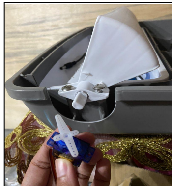
Figure 3.6.4: Installing The Servo Motor Using Hot Glue Gun
