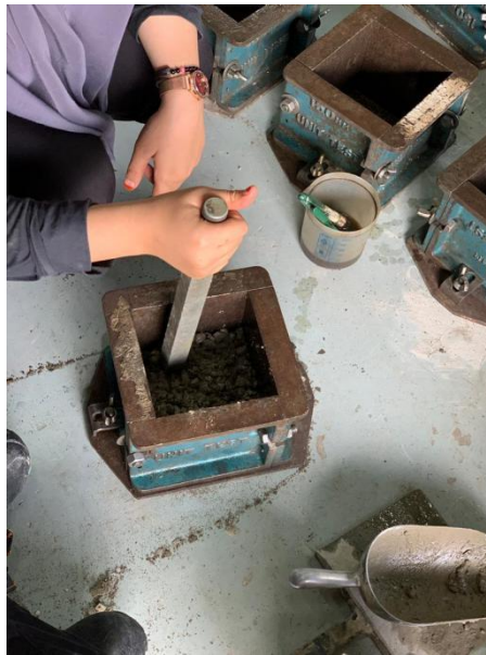
Figure 3.8 : The Mixture was Compacted
