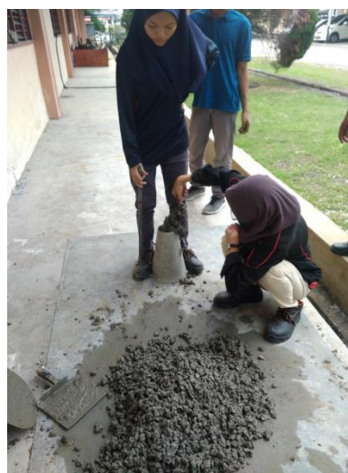
Figure 3.4 : Concrete Mixture Inserted into The Cone
