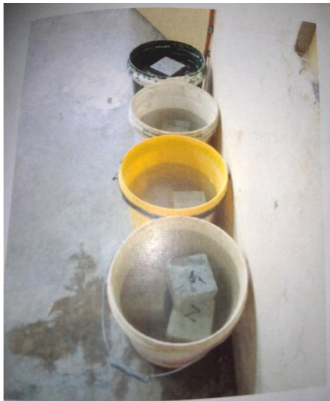
Figure 3.10 : The concrete soaked in the former
