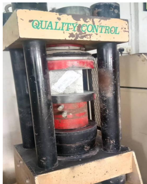
Figure 4.4 : The Concrete is Positioned at the Bottom of the Pallet
