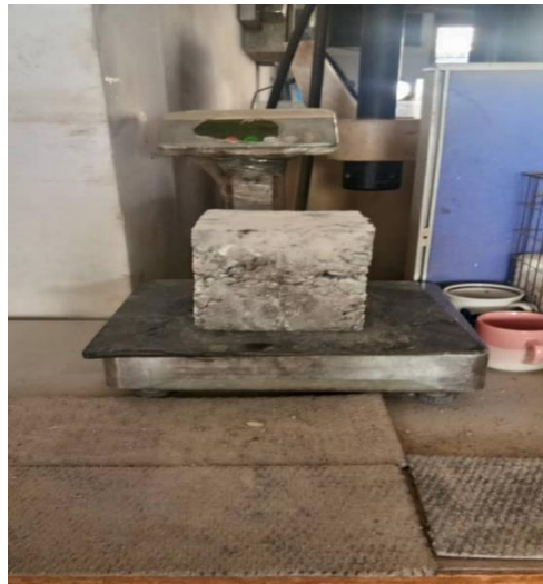
Figure 4.3 : Weight Concrete was Measured
