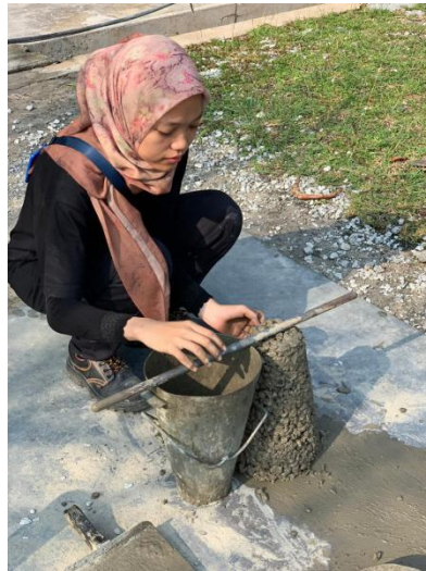
Figure 3.7 : The Collapse is Measured
