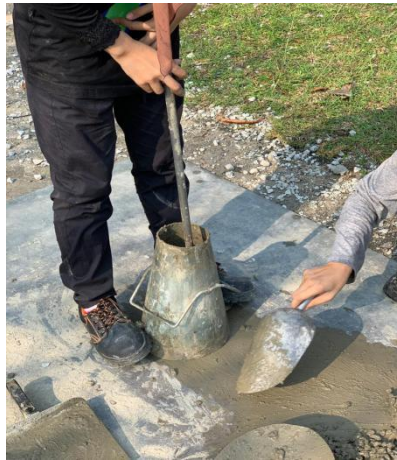
Figure 3.5 : Compacting Rod of 25 Times the Impact
